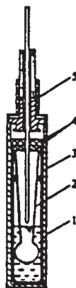
Fig. 1 Device used for the study of the formation reaction; 1 – calorimetric cell; 2 – adding tube containing sodium n -dodecylbenzene sulfonate solution or potassium nitrate; 3 – adding tube containing ceric(III) nitrate solution; 4 – silicone rubber cover; 5 – glass rod (on depressing the rod, the bottom of tube 2 is broken. The two solutions are mixed in the tube 1 and 2)
